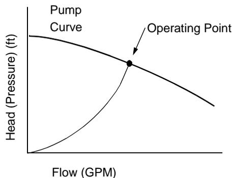
If the system is part of a process that requires adjustable flow rates, then some method is needed to continuously alter the pump characteristics or the system parameters. Methods include valves for throttling, which change the system curve, or variable speed control of the pump, which modifies the pump curve.
