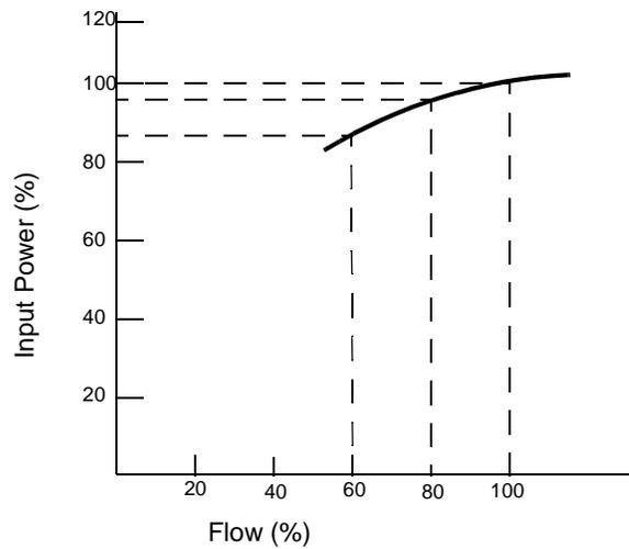
Inlet guide vanes direct the air flow as the air enters the fan, and, actually modify the fan curve (see the next figure).
