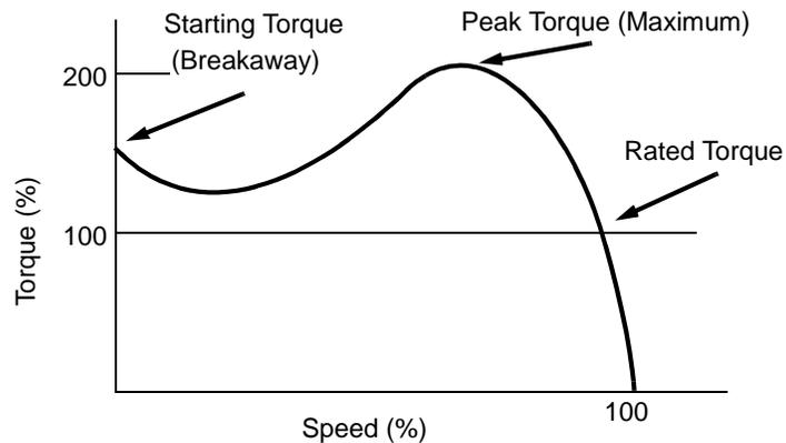
As seen in the figure, the torque produced at locked rotor (breakaway torque) is higher than rated torque, but less than the peak torque point.
