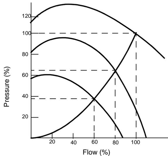
Using VFDs greatly reduces the power requirements, even more than for inlet guide vanes.(see figure below)
