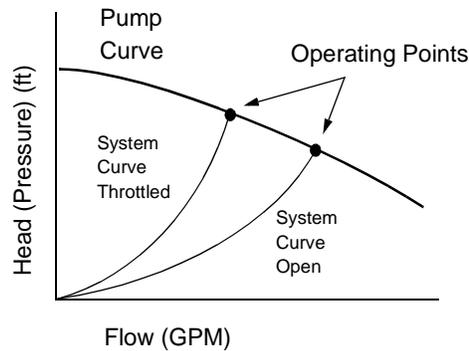
By comparison, the variable speed method changes the pump characteristics when the pump impeller speed is changed (see figure below).
