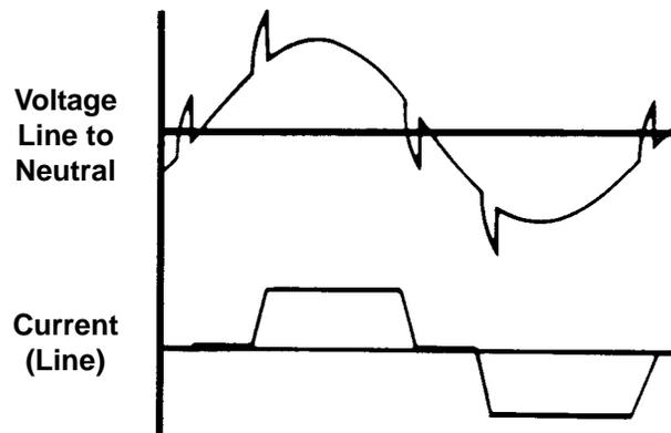
Figure AC-4. CSI Voltage and Current Waveforms
