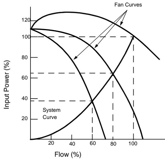
With these vanes, power requirements are significantly reduced as flow is decreased (see figure below).
