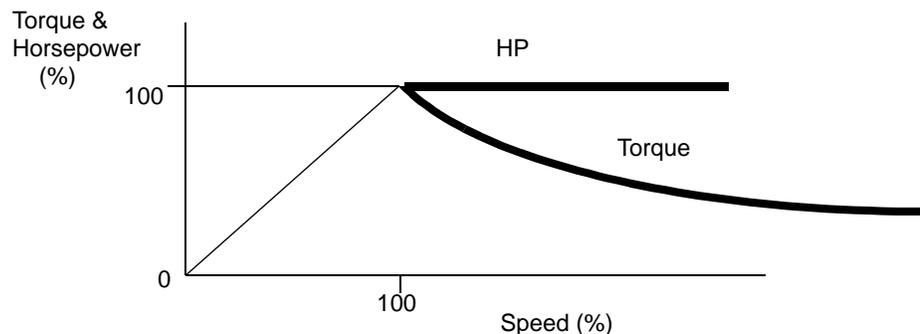
Examples of this type of load are center-driven winders and machine tool spindles. A specific example of this application would be a lathe that requires slow speeds for rough cuts and high speeds for fine cuts (e.g. little material is removed). Usually very high starting torques are required for quick acceleration.
