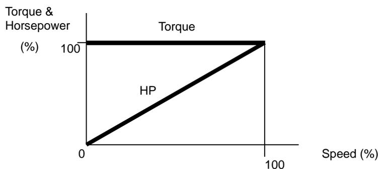
As shown in the figure, torque remains constant while horsepower is directly proportional to speed. A look at the basic horsepower equation also verifies this fact.
