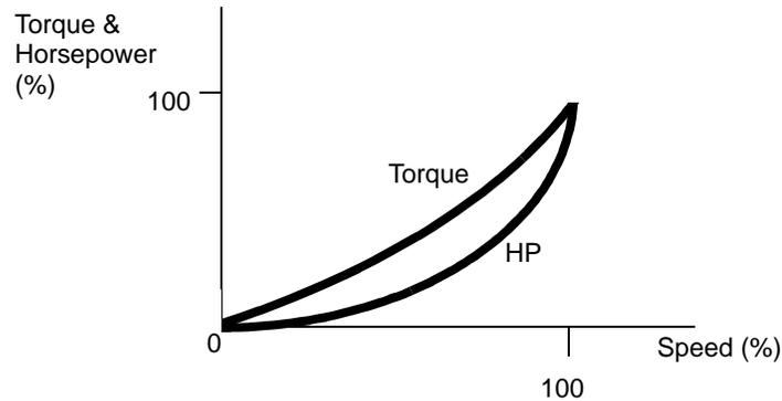
Examples of this type of load are centrifugal fans, pumps and blowers. This type of load requires much lower torque at low speeds than at high speeds.
