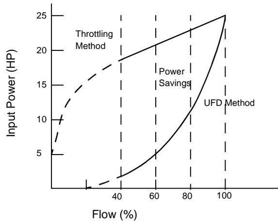
This example does not include a static head (pressure required to overcome a change in elevation). The magnitude of the static head will affect the possible power savings. The less the static head is in relation to the total head, the greater the power savings will be achieved by using VFDs--one with no static head, and two with different amounts of static heads.
