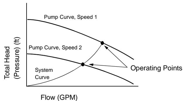
For a specific flow rate, the difference between points A and B gives a visual indication of possible energy savings (see figure below). In addition, changes in pump efficiency should be included in the calculation to determine brake horsepower.
