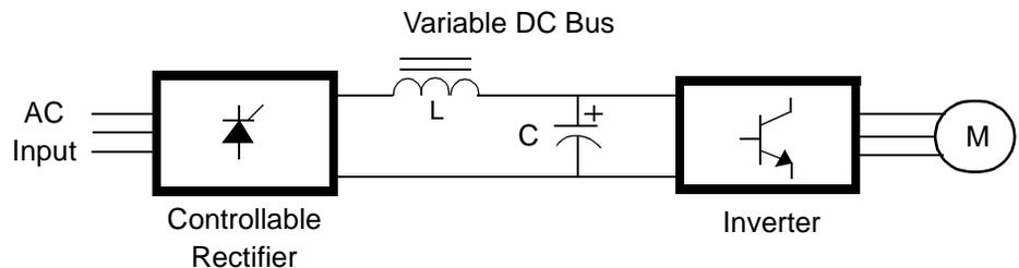
Figure AC-1. VVI Block Diagram
