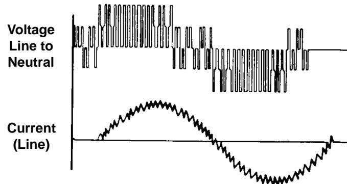
*Figure AC-6. PWM Voltage and Current Waveforms*
