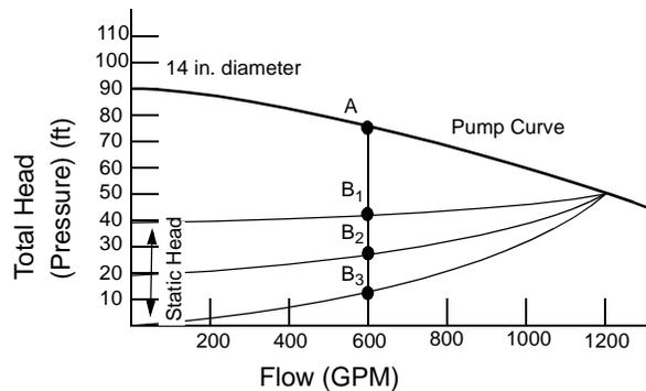
For a given flow rate, the difference between operating points A and B indicate possible power savings with VFDs. The difference between points A and B<sub>3</sub> (no static head) is greater -- and offers greater power savings -- than between a and B<sub>1</sub>, which has a 40 ft static head.
