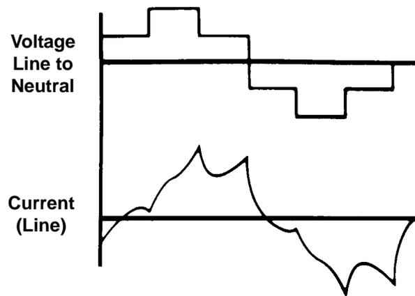
Figure AC-2. VVI Voltage and Current Waveforms
