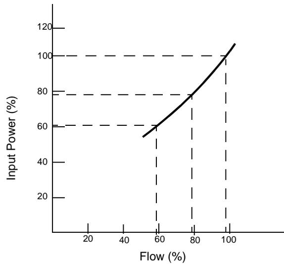
As with pumps, VFDs offer the greatest energy savings for fans. This adjustable flow method changes the fan curve (see the next figure).
